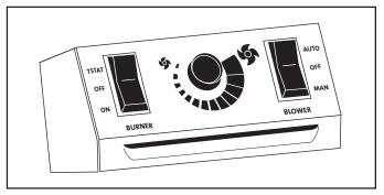
Figure 30. Burner Switch and Optional Blower Controls
